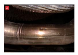
A) The original system requires cutting so it can be removed. We recommend using the original cutting point marked on the exhaust with indentations.
